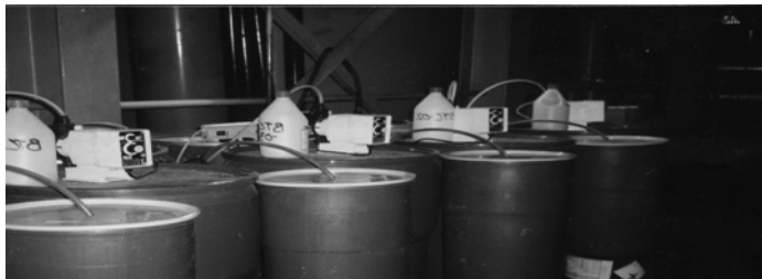
Column tests of cyanide degrading bacteria using various concentrations and growth conditions at the Brewery Creek Mine.
