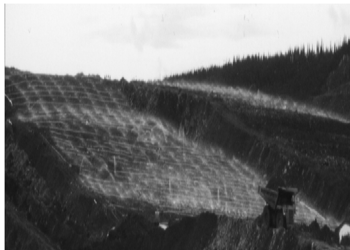
A weak cyanide solution sprayed onto a heap.
